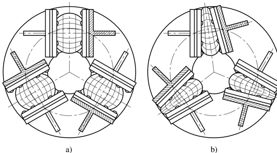
Figure 1. Tangential pneumatic flexible shaft coupling,
