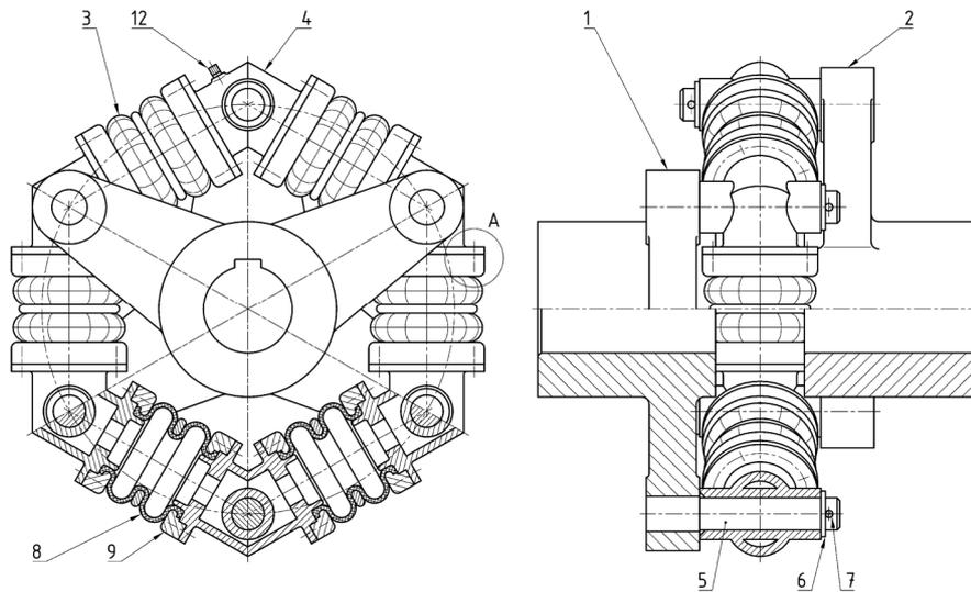
Figure 2. Tangential pneumatic flexible shaft coupling with axially deformed flexible elements – neutral position (unloaded coupling) [4]
