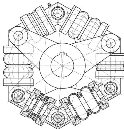
Figure 3. Tangential pneumatic flexible shaft coupling with axially deformed flexible elements – maximally deformed position (fully loaded coupling) [4]
