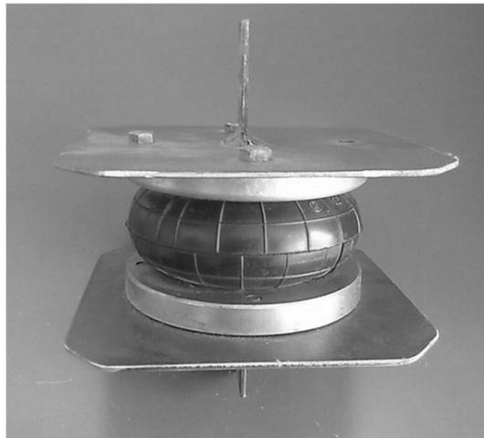
Figure 2. Pneumatic-flexible element with preparation
