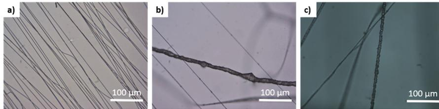
Figure 3. Microscopic images of PCL samples (a) pure PCL, (b) PCL with bioglass, (c) PCL with Zn\_bioglass
