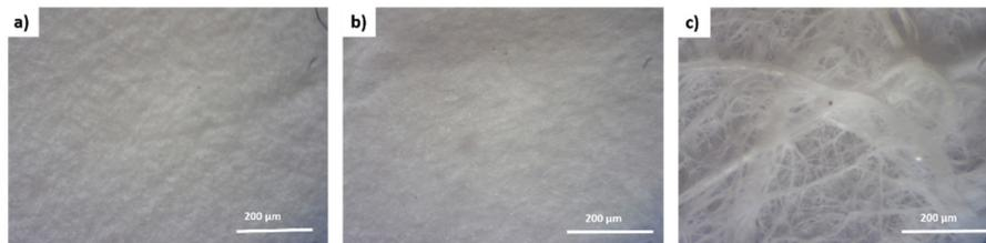
Figure 5. Macroscopic images of PCL samples after immersion in SBF (a) pure PCL, (b) PCL with bioglass, (c) PCL with Zn\_bioglass
