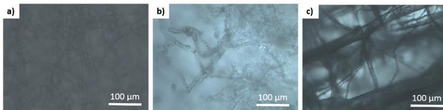
Figure 6. Microscopic images of PCL samples after immersion in SBF (a) pure PCL, (b) PCL with bioglass, (c) PCL with Zn\_bioglass
