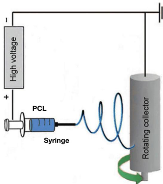
Figure 1. Scheme of electrospinning process.
