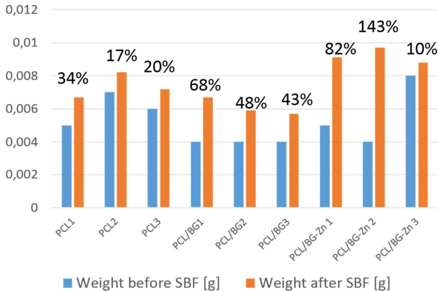
Figure 4. Weight change of samples after incubation in SBF fluid.
