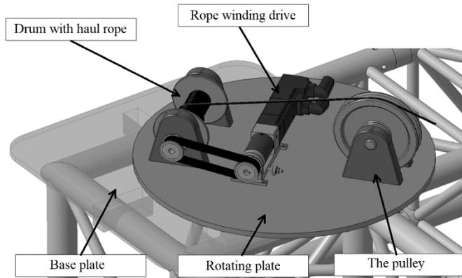
*Figure 5. Rope winding assembly*
