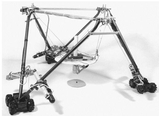
*Figure 1. Model of NIST RoboCrane[4]*
