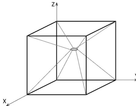
Figure 2. Working space of a Cable drive parallel robot with 8 haul ropes
