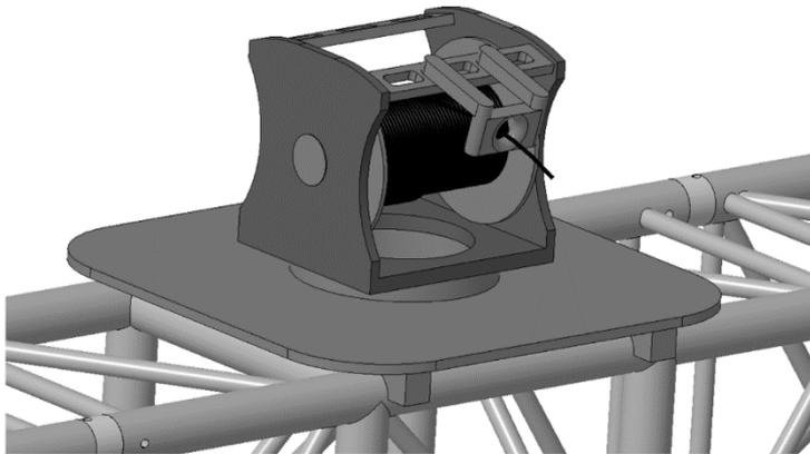
*Figure 6. Design of an automatic wiring machine*
