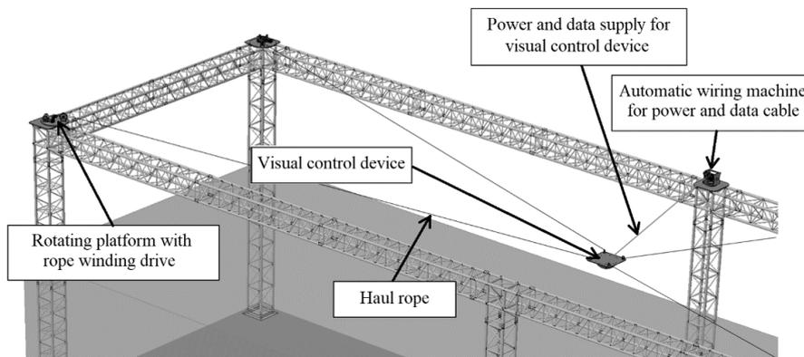
Figure 7. Assembly of the conceptual design
