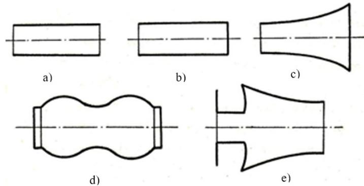
Figure 2. Various cylindrical shapes of flexible wheels
