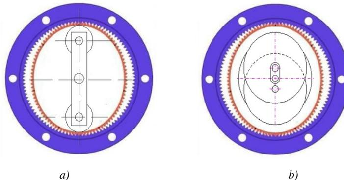
Figure 3. Deformation of harmonic gear;
