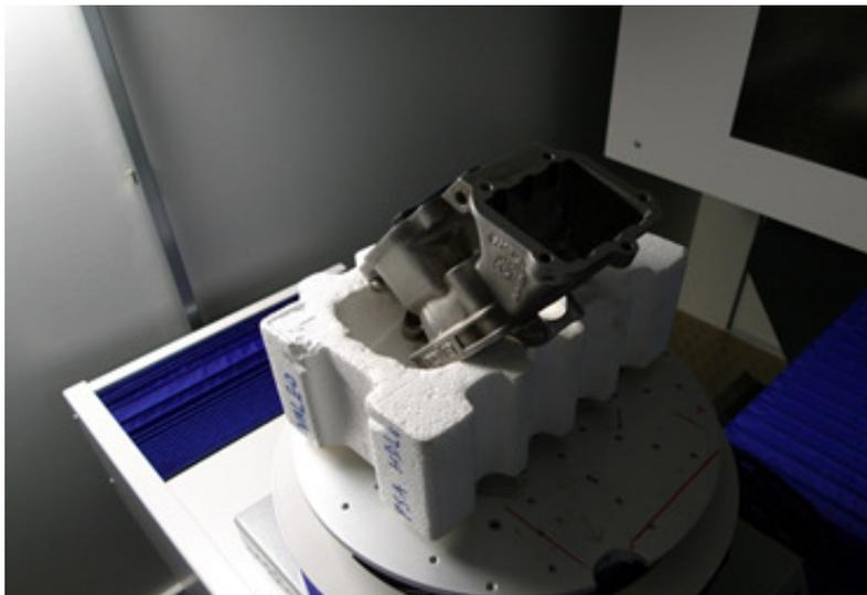
*Figure 7. Measuring the engine cylinder using a metrotome*
