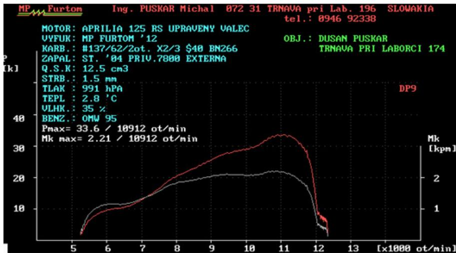
Figure 11. Performance and torque of engine with modified ignition
