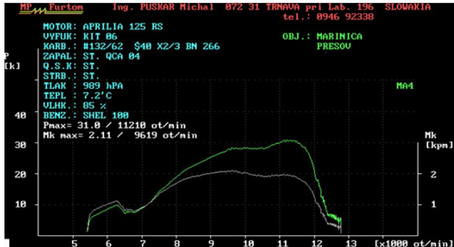
Figure 8. Performance and torque of untreated engine
