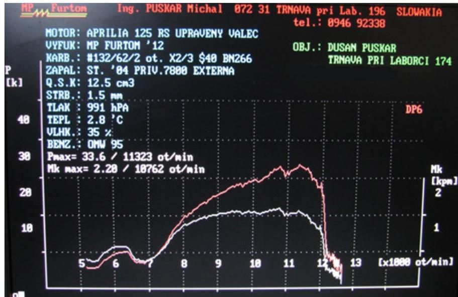
Figure 9. Performance and torque of modified engine
