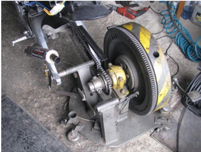
Figure 6. Measuring an experimental model on a power brake
