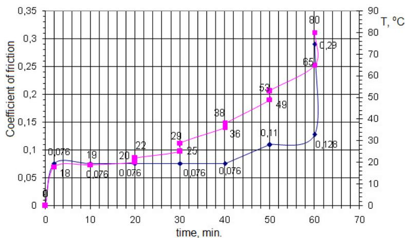
Figure 1. Graph of change of friction coefficient and temperature in the area of contact of tribosystem from time: ■ - the temperature; ◆ - the coefficient of friction
