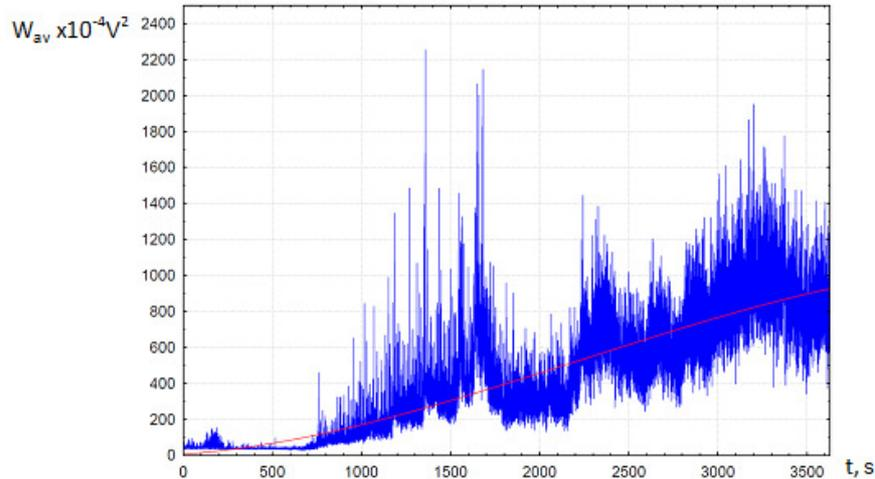
Figure 2. Dependence of change of the average power of AE signals in time (seconds), 30HGSA-D16 tribosystem
