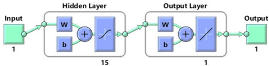
Figure 10. Feed forward neural network with 15 neurons in hidden layer
