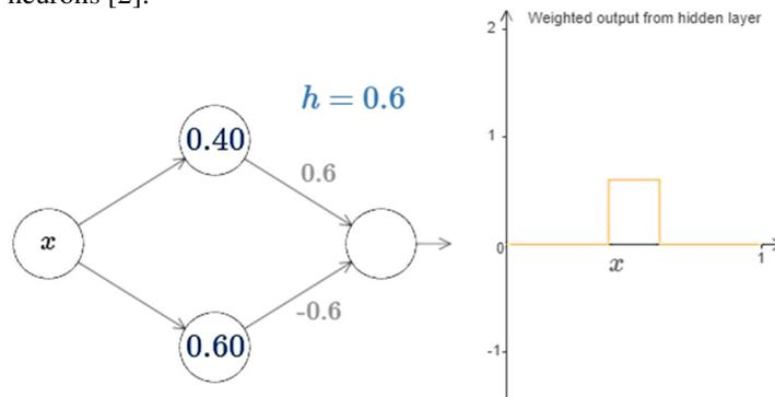
Figure 5. Simple tower function [2]
