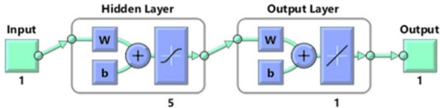
Figure 8. Feed forward neural network with 5 neurons in hidden layer
