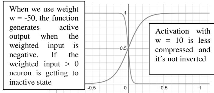
Figure 4. Impact of weight parameter on the output from neuron
