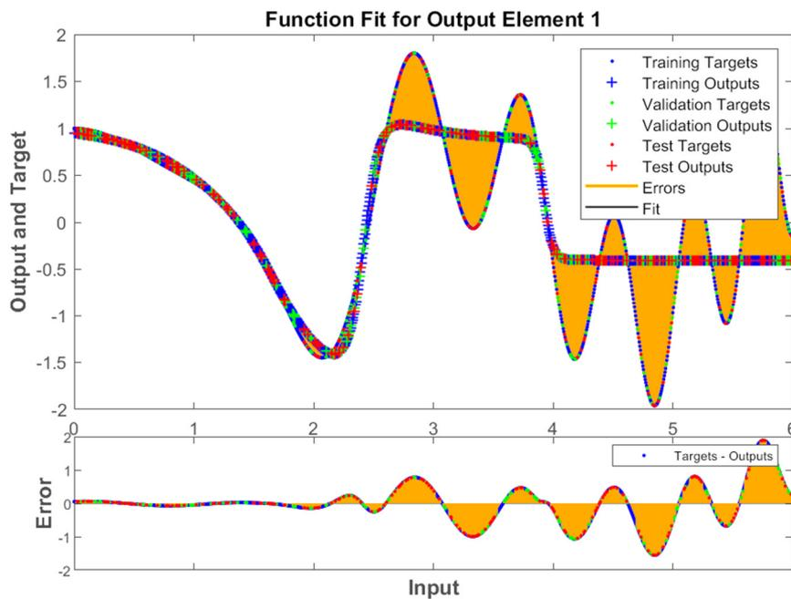
Figure 9. Approximation of the network with 5 neurons
