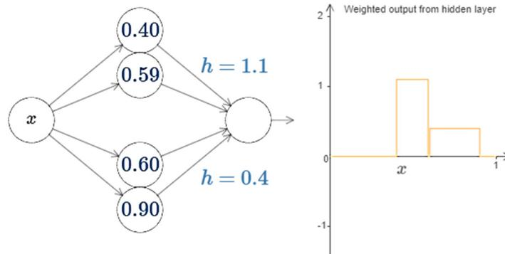
Figure 6. Tower functions from 4 neurons [2]
