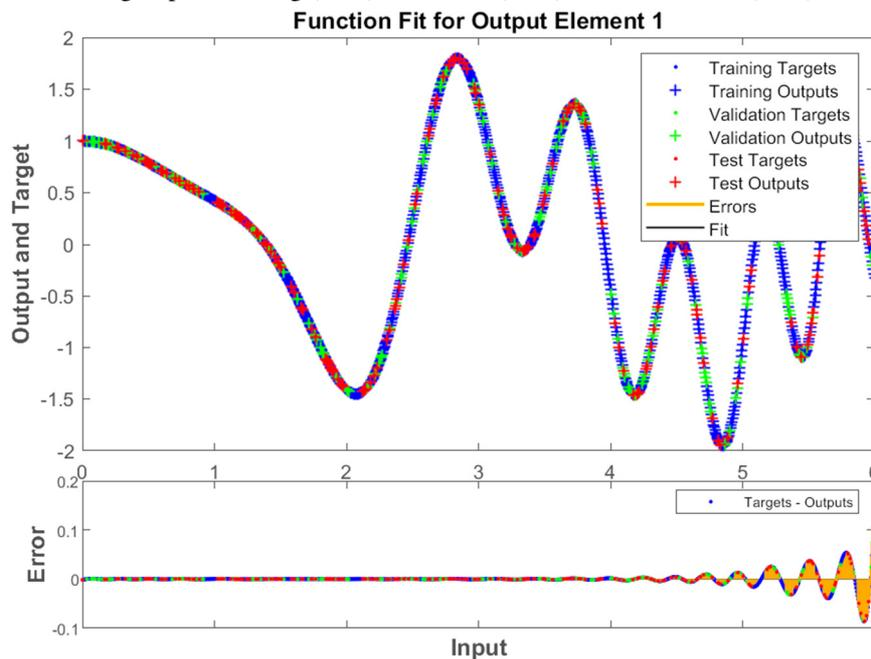
Figure 11. Approximation of the network with 15 neurons in hidden layer
