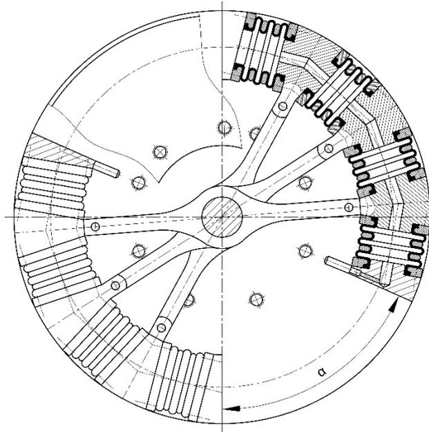
Figure 3. The tangential pneumatic flexible shaft coupling with serial arranged flexible elements in fully loaded state (at maximum twist angle  $\alpha$ )
