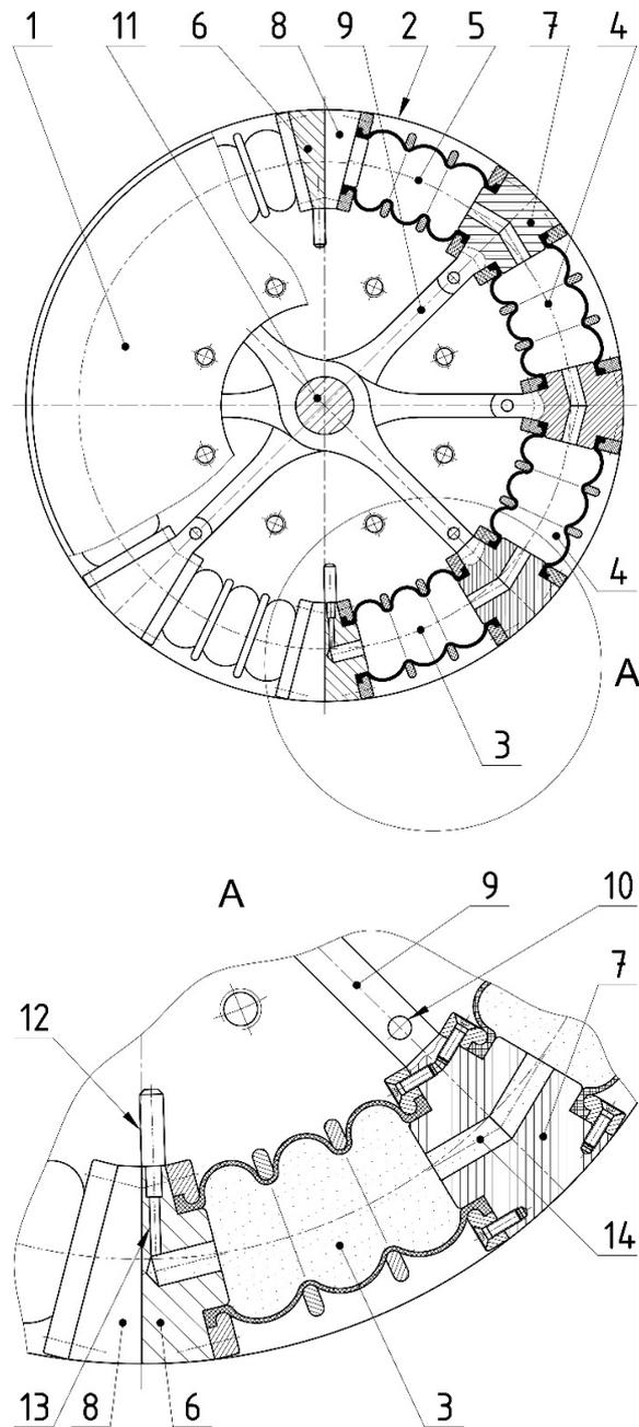
Figure 2. The tangential pneumatic flexible shaft coupling with serially arranged flexible elements in unloaded state
