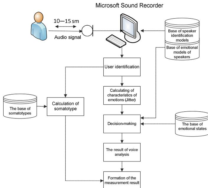
Figure 1. Functional diagram of the system of identification of insider features
