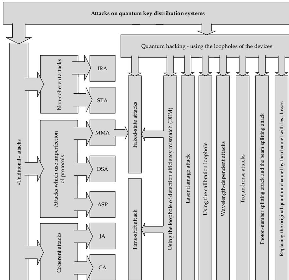
Figure 1. The extended classification of the methods of the eavesdropping and data corruption in the systems of quantum cryptography
