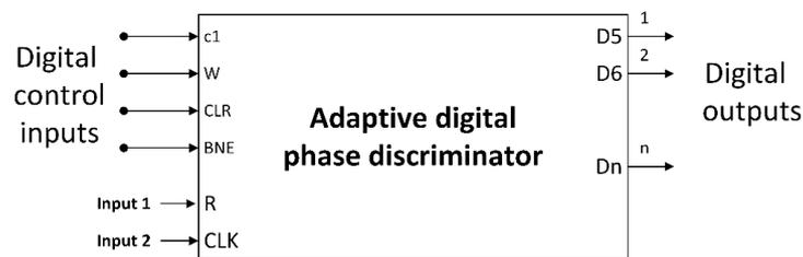
Figure 2. Scheme of adaptive digital phase discriminator
