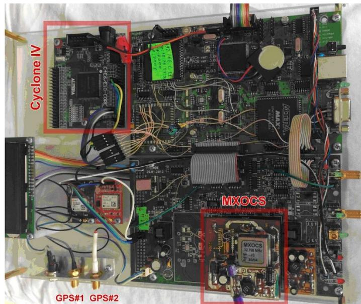
Figure 5. Laboratory stand MCDD AMS with two GPS receivers
