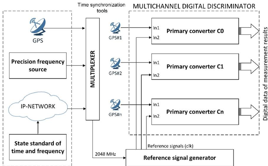
Figure 1. Scheme of the electric power networks SMART-GRID time synchronization monitoring automated system
