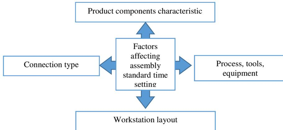
Figure 1. Factors affecting the standard time of an assembly process
