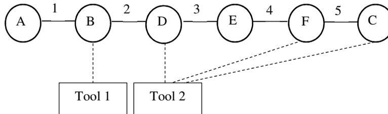
Figure 6. An example of an extended liaison graph (ELG)
