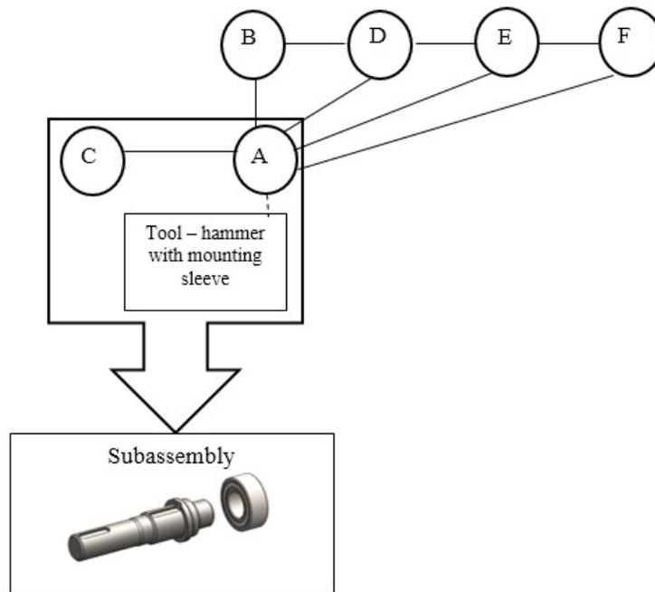
Figure 9. Subassembly analysed using ELG
