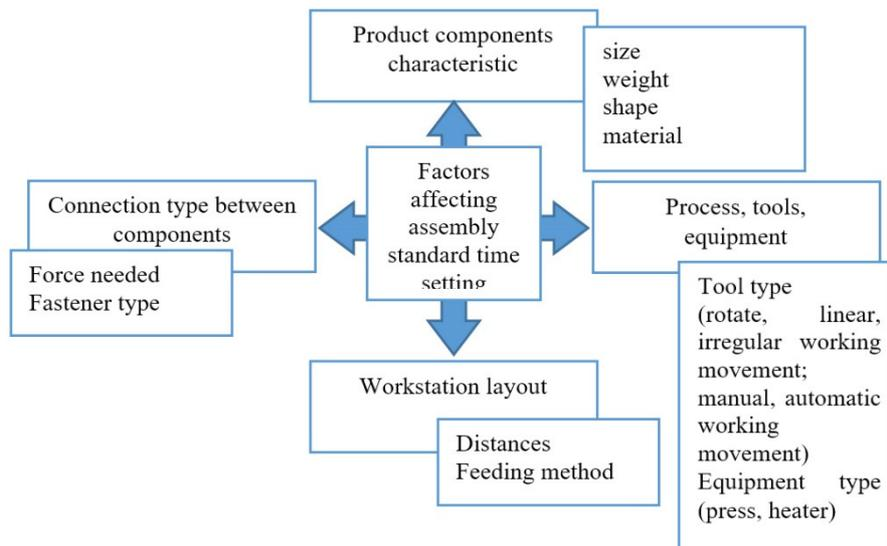
Figure 8. Factors (attributes) affecting standard assembly time of two components
