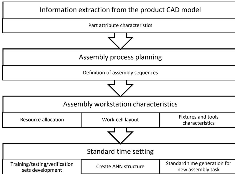
Figure 2. Standard assembly time setting in the early stage of product development for a mechanical product
