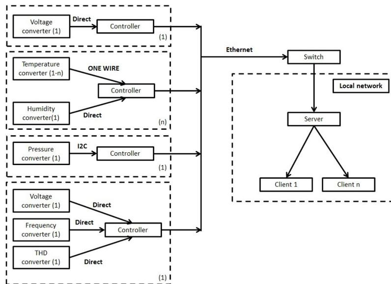
Picture 2 - The block diagram of an automated monitoring system
