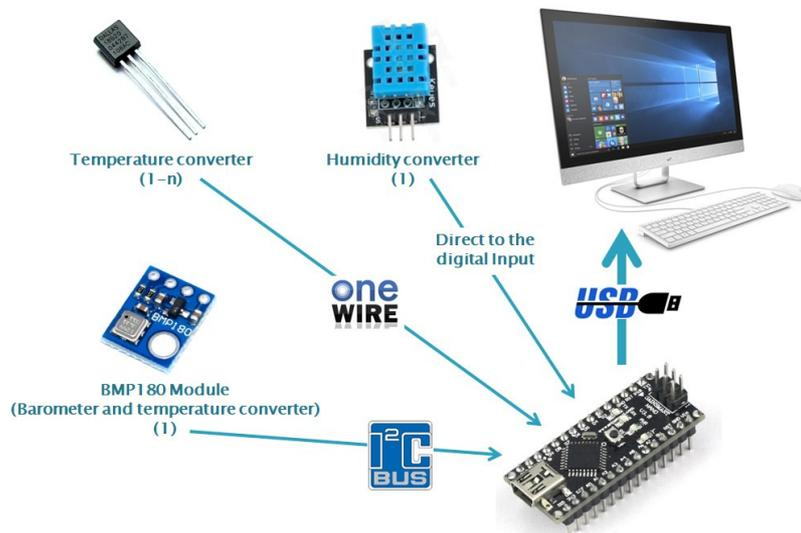
Picture 3 - Model of monitoring system
