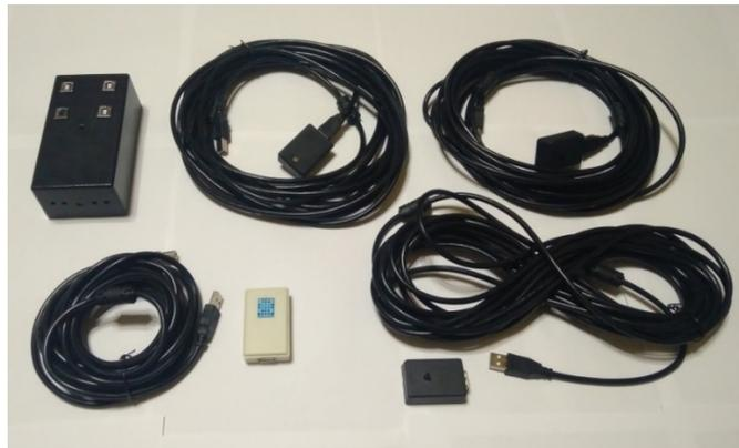
Picture 4 - Appearance of the prototype (without PC): from the upper left corner clockwise: a microcontroller with a module of pressure and temperature converter (this converter shows the temperature of the device), temperature converter (3 units) with adapters (10m), humidity converter with connecting conductor (5m).
