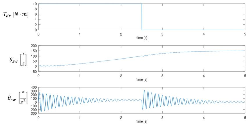
Picture 2. A driver's torque and the steering wheel angle's and angular velocity
