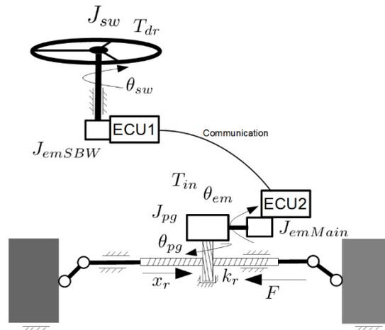
Picture 4. A sketch of the steer by wire EPS system
