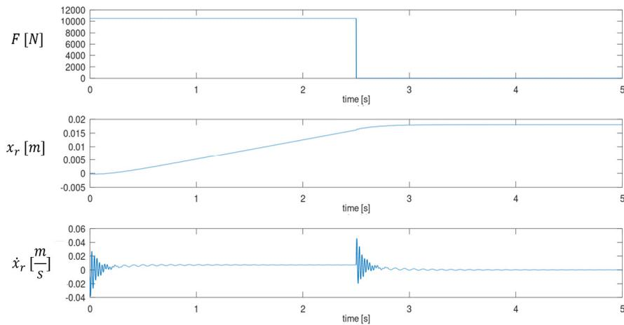
Picture 3. A force on rack and the rack's linear displacement and linear velocity
