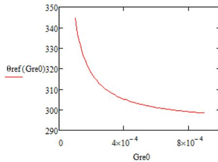
Figure 4. Static channel characteristic  $G_{re0} - \theta_{ref}$
