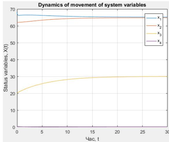
Figure 6. Transient characterization of the process by channels  $G_{r0} - \theta_{rf}$ ,
