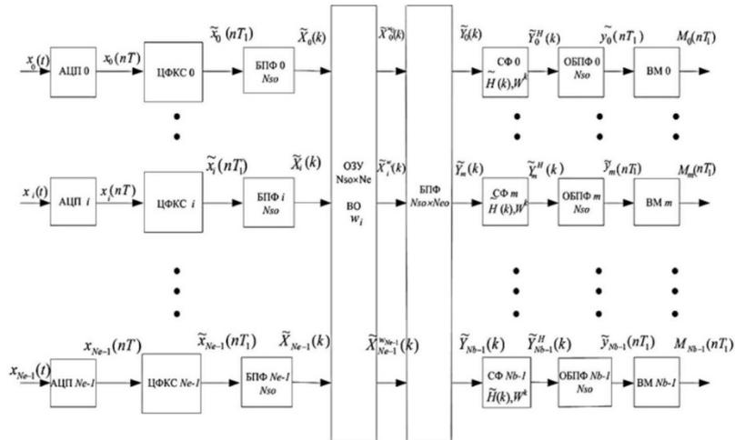
Figure 3. Formation of directivity characteristics in the frequency domain
