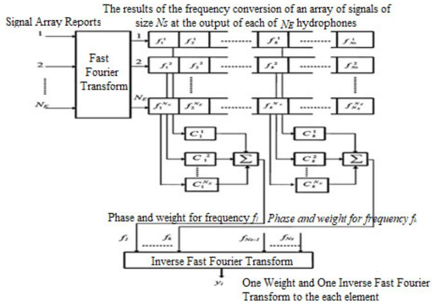
Figure 2. Algorithm for the formation of directivity characteristics in the frequency domain.
