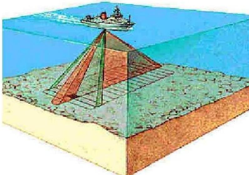
*Figure 1. Multipath Echo Sounder Operation.*
