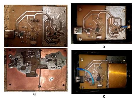
CYWUSB6935-Based LPT Analyzer and CYWUSB6935-Based USB Analyzer
