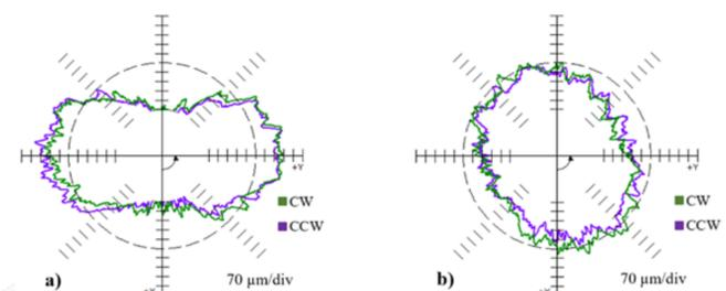
Figure 3. Circular path profile before (a) and after (b) robot calibration
