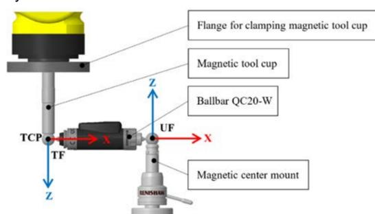
Figure 1. Measuring assembly and location of coordinate systems
