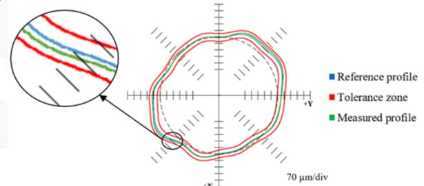
Figure 4. Polar graph with a reference profile for industrial robot status monitoring
